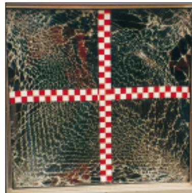
**Window with FrameGard™ and Madico™ security window film after a blast - The glass has been held securely in place.**
