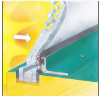
**Step Three:** Madico FrameGard™ movement zone absorbs energy by allowing window film to stretch. Radiused edge prevents cutting of film. Gripped surface clamps film in place.
