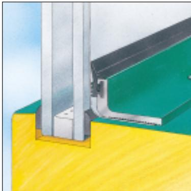
**Step One:** Madico FrameGard™ secures the film tightly in place to the window frame.
