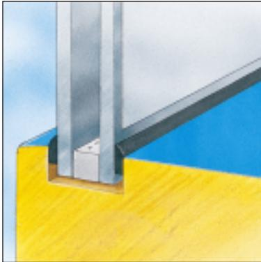
**Step One:** Daylight window film with gap shown around edge.
